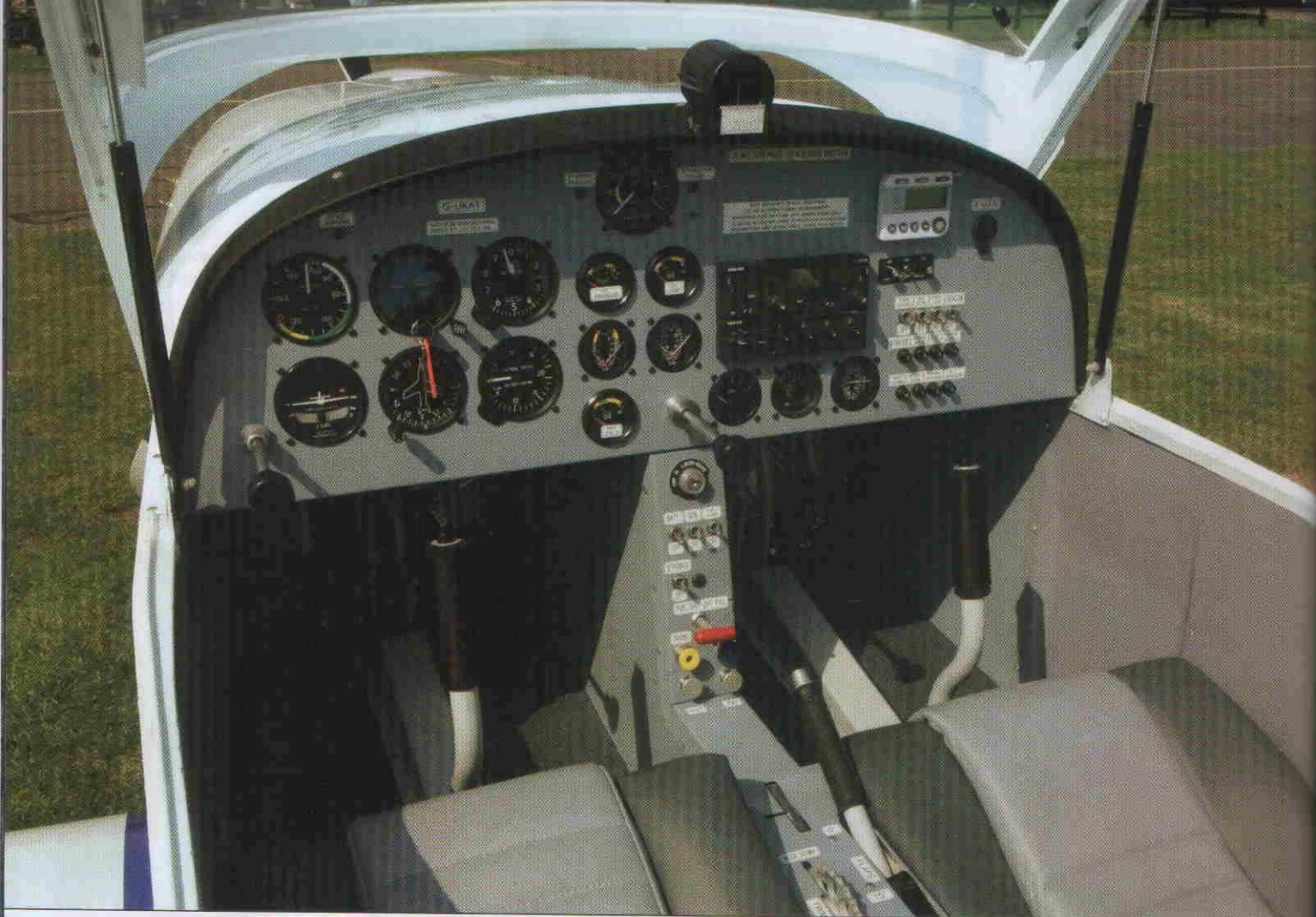
Basic finish is what you might expect in a trainer: proper sticks may spoil students progressing to Cessnas & Pipers, those 'self-opening' Rotax throttles will not!
