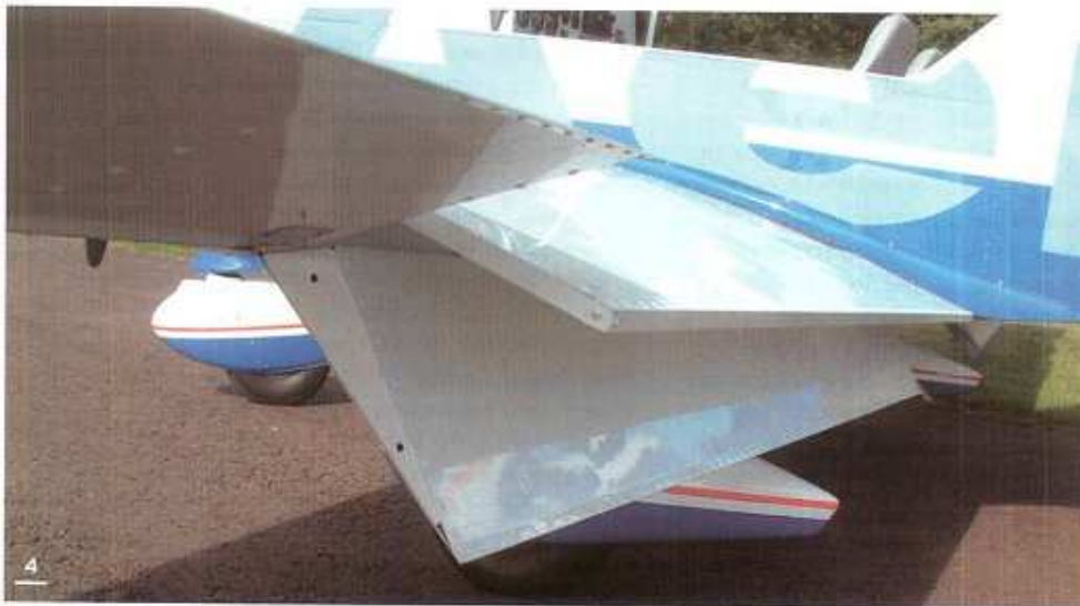
4 | Split flaps produce more drag than conventional simple flaps, as well as up to ten per cent extra lift. Ailerons are relatively small but still have good authority.
